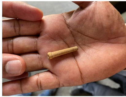
Figure 34: Metallic filter inside the humidifier connector valve
