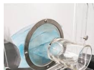
Figure 3: Mask synthetic blood penetration tester
